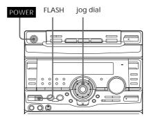
/ Press and hold FLASH during playback at the point you want to start the Flash function, and release to resume normal play.
